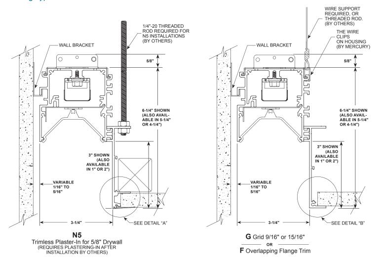
**NOTE:** Fixture must be installed prior to ceiling in all drywall applications (N5 and F).
