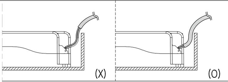
※ The cable protective sheath should be removed only near the terminal block to ensure that the exposed base insulation wire does not touch the surrounding metal.
