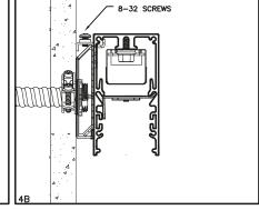
STEP 4: HANGING THE FIXTURE: 4A-RAISE UP FIXTURE A FEW INCHES ABOVE THE WALL MOUNT BRACKET. PROCEED WITH DOWNWARD ROTATING MOTION, REST FIXTURE ON WALL MOUNT 4B-TIGHTEN 8-32 SCREWS ON HOUSING BRACKET UNTIL FIXTURE IS SECURED.
