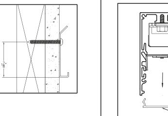
STEP 2: -REMOVE LENS FROM EACH 'STARTER', 'MIDDLE' AND 'END' FIXTURES. -MARK EACH LENS TO CORRESPONDING FIXTURE TO BE REINSTALLED IN STEP 7.
