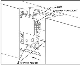
STEP 5: -HANG THE MID/END FIXTURES AS SHOWN IN STEP -ALIGN FIXTURE USING ALIGNERS BY MERCURY -CONNECT POWER CONNECTOR BETWEEN FIXTUES.
