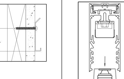
STFP 2: -REMOVE LOUVER FROM EACH 'STARTER', 'MIDDLE' AND END FIXTURES.
