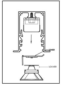
1A-REMOVE LOUVER AND COVER/LED BOARD MOUNT TRAY FROM FIXTURE(S).
