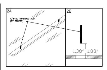
2A-VERIFY THAT 1/4-20 THREADED ROD FROM STRUCTURE ABOVE IS AT THE CORRECT LOCATION
