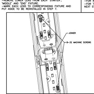
PUSH EXCESS POWER CONNECTOR CABLES BACK INTO FIXTURE THROUGH JOINERS AS SHOWN FOR MLS-2 OR TO EITHER SIDE OF JOINER FOR MLS-3 -SECURE FIXTURES TOGETHER USING (2) 8-32 SCREWS THROUGH JOINER AS SHOWN ABOVE (PROVIDED BY MERCURY). -REPEAT STEP 4 & 5 AS NEEDED UNTIL 'END' MODULE IS INSTALLED.
