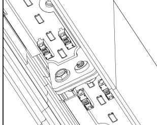
COMPLETE JOINT ASSEMBLY -ONCE FINAL LEVELING IS COMPLETED, CUT OFF EXCESS CABLE AND LEAVE 1/2" COMING OUT FROM CABLE GRIPPER AS SHOWN.(SEE DETAIL 2A ABOVE) -AIRCRAFT CABLE MANUFACTURER RECOMMENDS A DAB OF CRAZY GLUE ON CUT CABLE TO AVOID UNRAVELLING.(SEE DETAIL 2A ABOVE)
