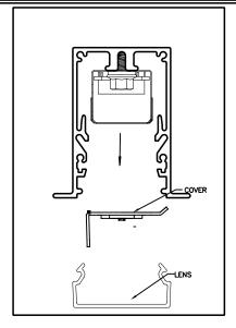
1A-REMOVE LENS AND COVER/LED BOARD MOUNT TRAY FROM FIXTURE(S)
