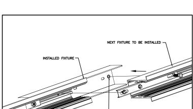
1/4-20 PEM NUT ON EXTERNAL JOINING BRACKET-
