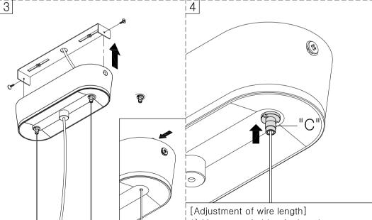
After lifting the flange, fix the bracket
