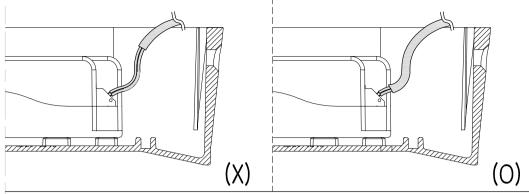
\* The cable protective jacket have to be removed only near terminal block to ensure uncovering basic insulation wire not touch the metal around.
