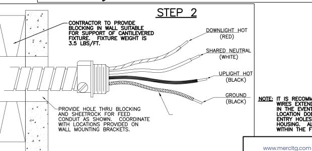
NOTE: IT IS RECOMMENDED THAT SUPPLY WIRES EXTEND 24" FROM CONNECTOR IN THE EVENT THAT THE FEED LOCATION DOES NOT ALIGN WITH THE ENTRY HOLES PROVIDED IN FIXTURE HOUSING. ALL SPLICES MUST OCCUR WITHIN THE FIXTURE HOUSING.
