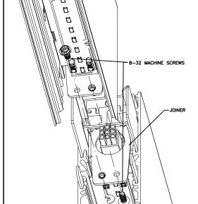
PUSH EXCESS POWER CONNECTOR CABLES BACK INTO FIXTURE THROUGH JOINERS AS SHOWN FOR MLS-2 OR TO EITHER SIDE OF JOINER FOR MLS-3 -SECURE FIXTURES TOGETHER USING (2) 8-32 (PROVIDED BY MERCURY).
