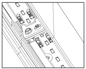
COMPLETE JOINT ASSEMBLY -ONCE FINAL LEVELING IS COMPLETED, CUT OFF EXCESS CABLE AND LEAVE 1/2" COMING OUT FROM CABLE GRIPPER AS SHOWN (SEE DETAIL 2A ABOVE) -AIRCRAFT CABLE MANUFACTURER RECOMMENDS A DAB OF CRAZY GLUE ON CUT CABLE TO AVOID UNRAVELLING.(SEE DETAIL 2A ABOVE)
