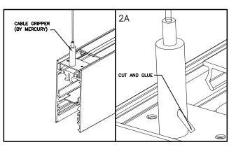
STEP 2: -START WITH INDIVIDUAL/STARTER MODULES BY INSERTING AIRCRAFT CABLES INTO CABLE GRIPPERS -ADJUST CABLE UNTIL FIXTURE IS AT CUSTOMER'S SPECIFIED HEIGHT AND LEVEL.
